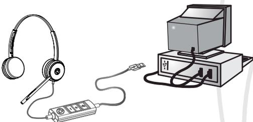
The Bravo USB does not require the installation of additional software or drivers. Plug the USB connector to one of the USB ports of the PC. The system will recognize the connection of your headset and from then on, all multimedia functions will be performed by the headset.
