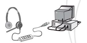
Epko X USB does not require the installation of additional software or drivers. Plug the USB connector to one of the USB ports of the PC. The system will recognize the connection of your headset and from then on, all multimedia functions will be performed by the headset.
