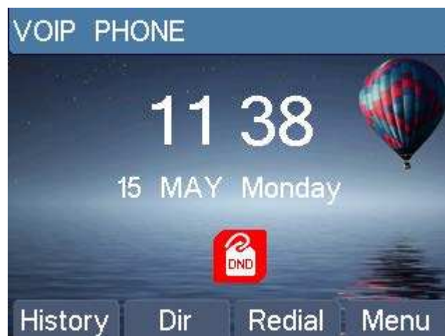
Figure 56 - DND Enabled on All Lines
